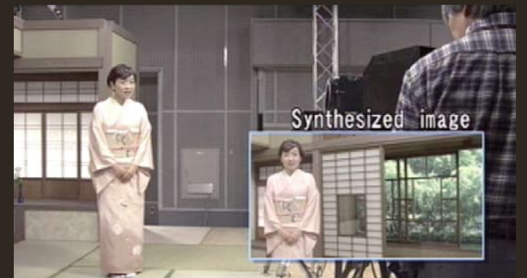
In a virtual studio using the camera, a woman appears to vanish into a prerecorded image of a sliding door.
